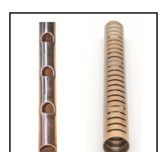
Our punch machines all produce flat holes, punching from the outside to the inside of the tube. There are many advantages to this process of hole-making, the two most important are speed and cleanliness. This process produces a slug as waste rather than chips, no lubricant is required. These machines are fast and accurate.
